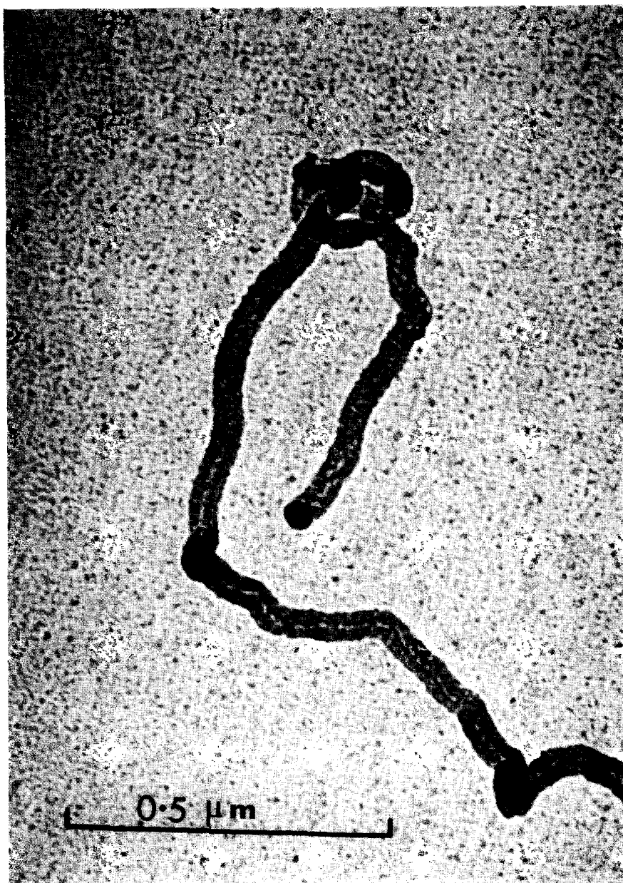
FIG. 2. Micrograph of a filament showing "pear-shaped" catalyst particle at its head. \times 120,000 .
